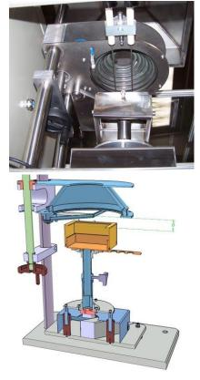
The system derives do not exceed 1 g in 30 minutes (evaluated during calibration).
