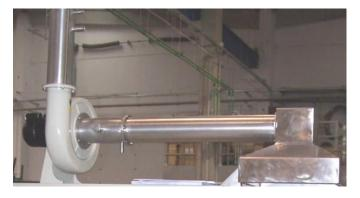
Inside the extraction system, it is placed an orifice of  $57 \pm 3$ mm diameter between the duct and the hood for the flow measurement.
